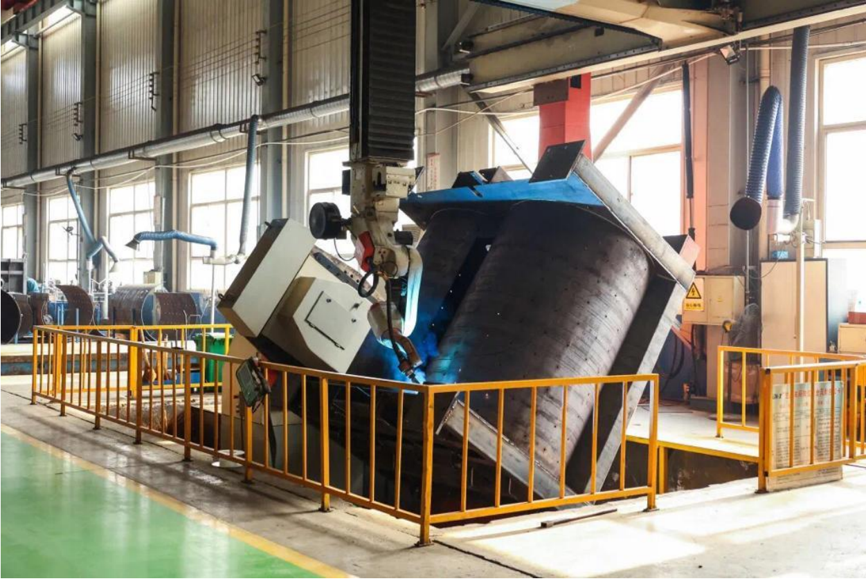
*Tam otomatik, Avusturya menşei IGM Kaynak Robotu / IGM brand fully-automatic welding robot with Austria origin
